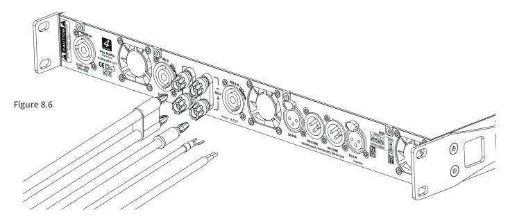
Select the appropriate size of wire based on the distance from amplifier to speaker.
