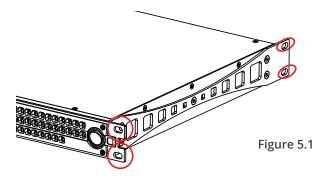
The common installation of the SX-Amplifier Series is in 19" standard rack cabinets. In order to limit the risk of mechanical damages, the amplifiers must be fixed to the rack using both frontal and rear mounting brackets. (See Figure 5.1)
